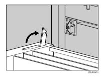
Hook the hole of the auxiliary bar onto the printer's mounting bracket.
