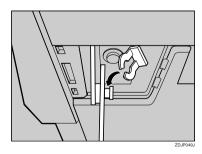
Make sure the auxiliary bar and stopper are installed in the positions, as shown.
