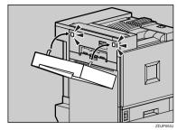
Remove the adhesive tape holdings the cable, and then connect the cable from the duplex reversal unit to the upper connector on the back of the printer.
