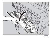
2 Remove the two small covers by pinching and pulling them in the direction of the arrow.
