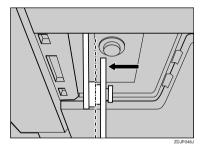
In step [5], move the auxiliary bar to the position with the perforated line, as shown.
